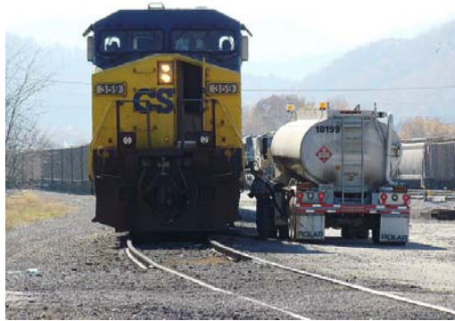
Figure 3. Example of Direct Truck-Locomotive (DTL) fueling operation for a locomotive.
